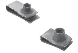
**Flat Nuts:** Made of spring steel and used where the other side of the panel is easy to reach. They can be for either stud type or threaded fasteners. They are used throughout the car under the dashboard, in door panels, trunk area, fenders, etc.
