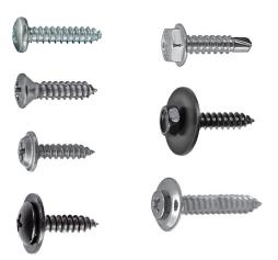
**Teks**: A screw with a drill point that drills its own hole as it is installed. Most Auveco Teks screws have a #2 point which is recommended for material up to .110" thick. The higher the drill point number, the thicker that material it can drill though. Once the metal is penetrated, the Teks fastener functions as a conventional tapping screws.
