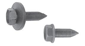
**Bumper Bolts:** Used to attach bumpers. They have either a USS coarse or metric regular pitch thread. Bumper bolts are usually zinc plated with a stainless steel capped head.
