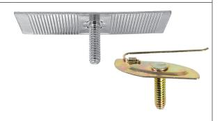
Washer Head: A screw/bolt with the washer permanently attached to it. Also called flanged head. The washer head eliminates the need for a separate washer while increasing the load bearing area of the head. Used under the hood, on fenders, doors, front end applications, etc.
